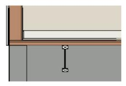
8. Using this technique, you can set the floor joist so that its top is flush with the top of the stem wall, and then make copies of that joist for the rest of the plan.
