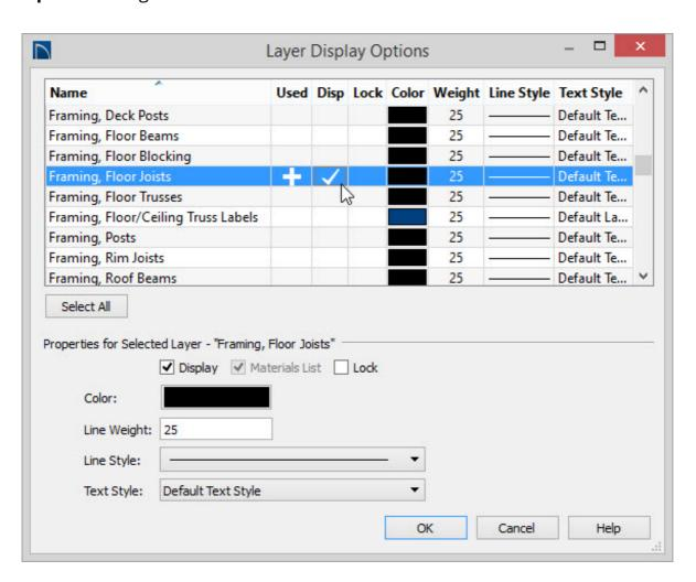
3. Once this dialog is open, put a check in the **Disp** column next to the "Framing, Floor Joists" layer to allow the floor framing to be displayed in the 3D view. Click the **OK**
