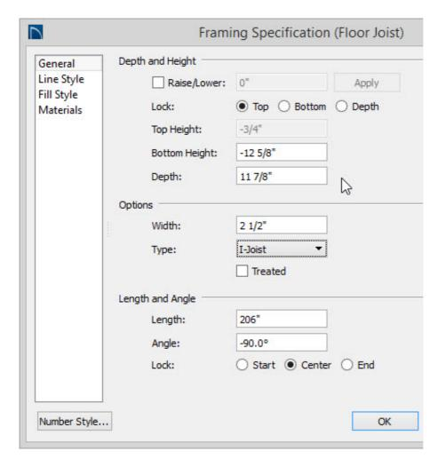
• On the General panel, click in the **Depth** field and change this value to the thickness of your joist then click **OK**.
