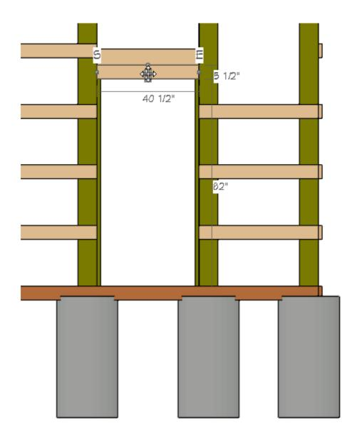
4. Select the top-most girt on the left side of the wall and use its edit handles to extend it to the outside of the corner pole on the right.
