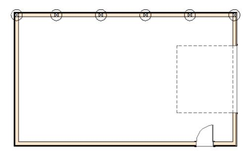
10. Repeat the steps above as needed to produce posts with footings around the perimeter of the structure.
