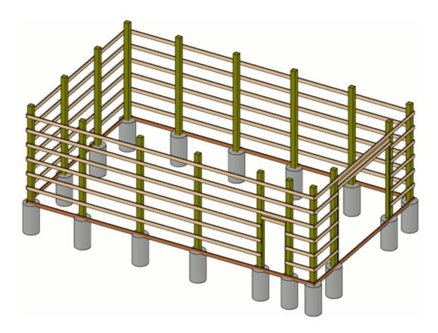
As part of the process of drawing the girts, the horizontal door furring has been created. Vertical furring should also be added.
