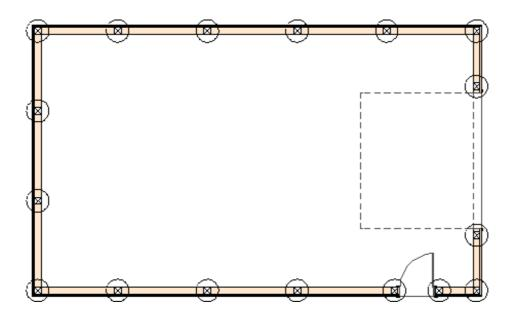
13. Select **Build> Floor> Build Foundation** I from the menu, then click **OK** to build a monolithic slab foundation using the default settings that were created earlier.
