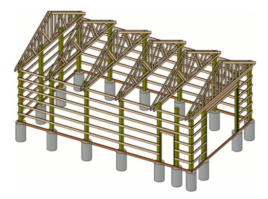
Both upper and lower blocking for the roof trusses can now be created.
