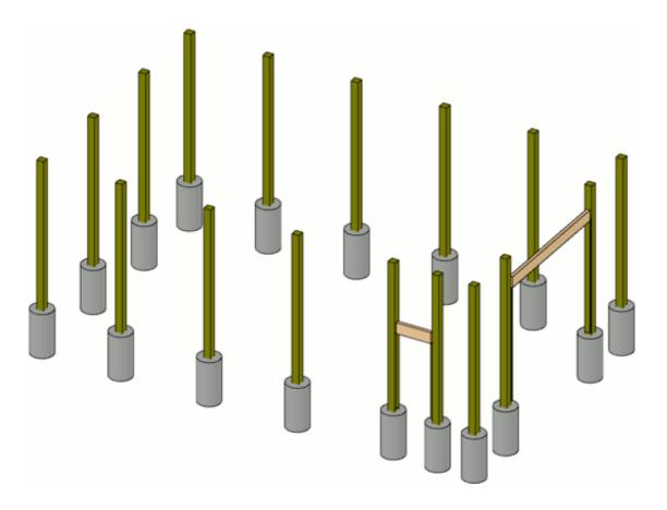
Once the poles and door framing is complete, girts can be added. The base girts can serve as the form for the concrete floor if you wish.
